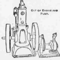
for Simplicity it Beats the World. It oils itself from a Reservoir, No Carburetor to get out of order. No Batteries or Electric Spark. t runs with a Cheaper Grade of Gasoline than any other Engine.
