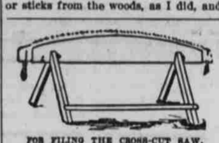
FOR FILING THE CROSS-CUT SAW.
