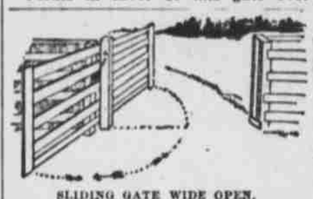
SLIDING GATE WIDE OPEN.
