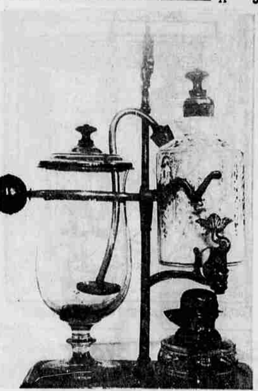
The contraption pictured above is one of the original vacuum-type coffee makers. Probably few realize that this method was invented in 1840 by a Scotsman, Robert Napier, a marine engineer, who turned his attention from ships to coffee-pots and built this elaborate machine. The accompanying article relates the history of coffee making and principle of Mr. Napier's invention.
