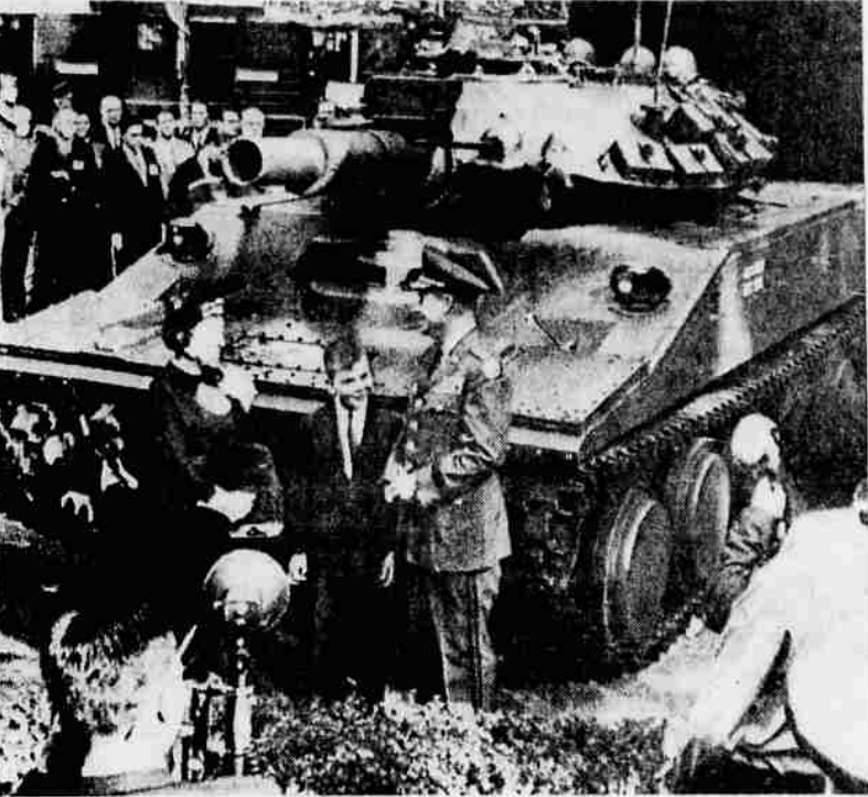
NEW TANK UNVEILED — The General Sheridan, the Army's new armored reconnaissance vehicle, is unveiled at the Association of the U.S. Army's annual meeting in Washington. Designed to provide troops with an armored reconnaissance and air-droppable assault vehicle, the General Sheridan will be able to fire both the Shillelagh surface-to-surface
