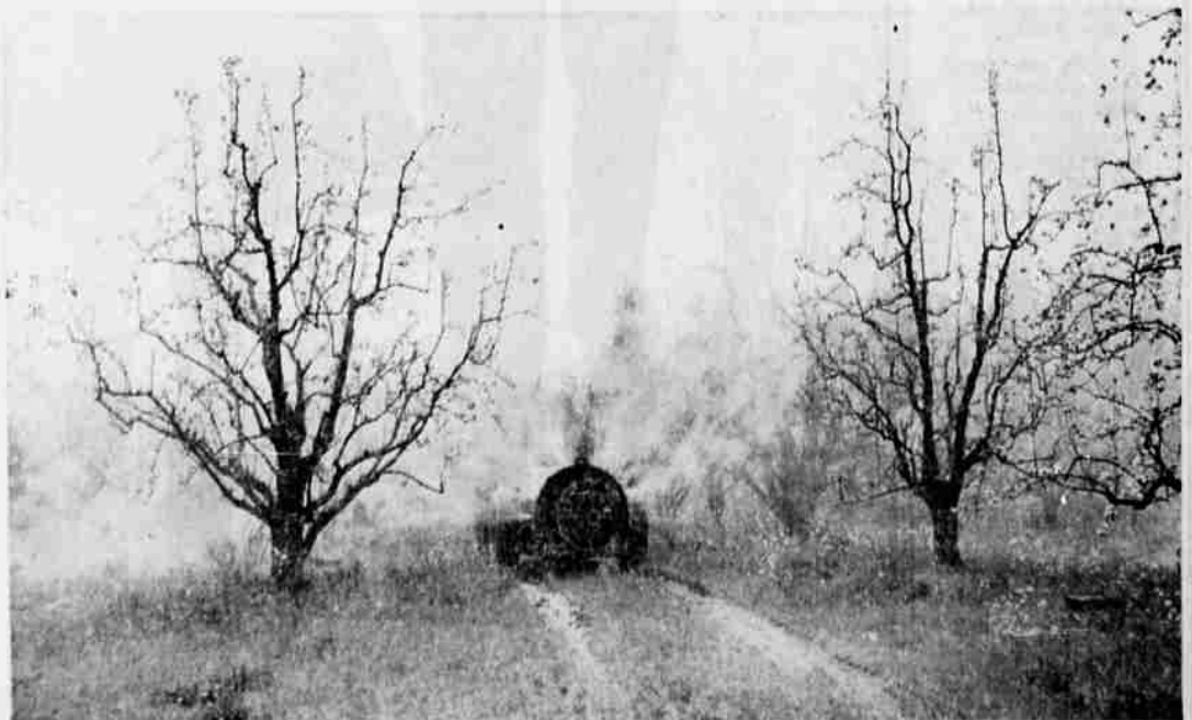
This is the airblast sprayer commonly used in orchards today. All it requires in the way of man-power is someone to drive the tractor. (Knackstedt Photo)
