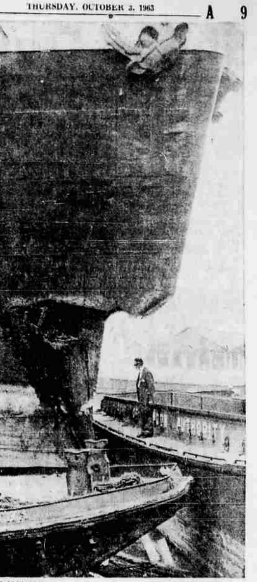
NOT MONSTER'S JAWS —This investigator seems to have wandered into the jaws of some prehistoric monster. He is inspecting the severely damaged bow of the British steamer "Mary Queen" which was in collision with the Dutch motor vessel "Vanguard" near London. The "Vanguard" sank and the British ship picked up the 11 members of her crew. (UPI)
