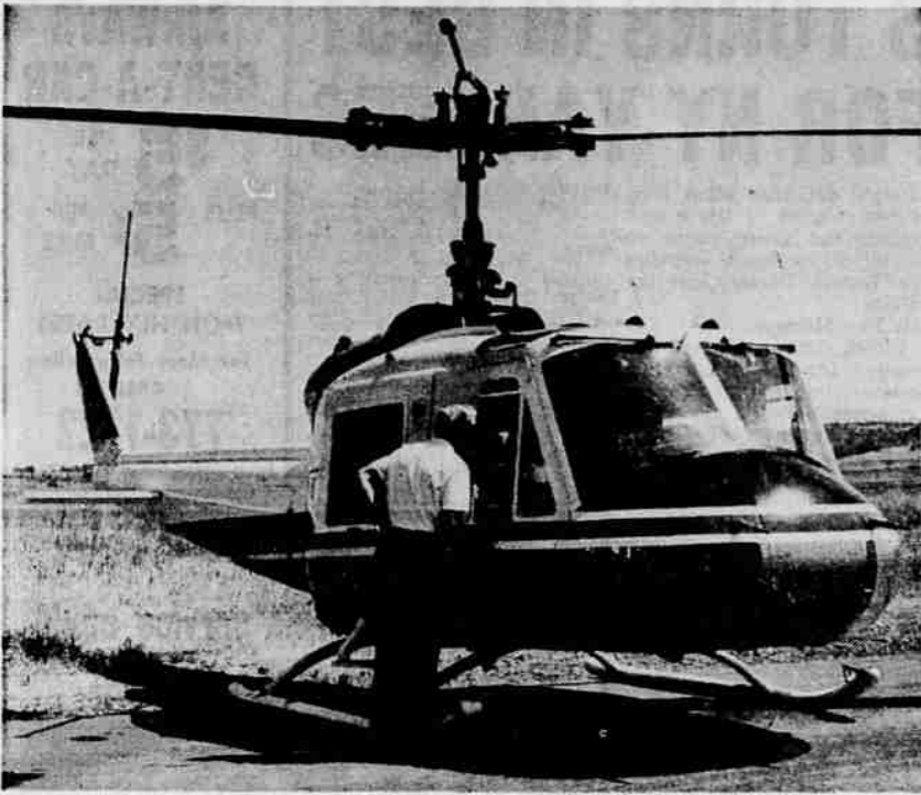
HELICOPTER STOPS HERE — Bell Helicopter company's Model 204B stopped at the Medford airport yesterday while on a western demonstration tour. The aircraft with a carrying capacity of 10 to 12 passengers and useful load of 3,182 pounds with seats removed is the largest helicopter Bell has in production. Its gas turbine engines can put it in the air and a mile away in 30 seconds.
