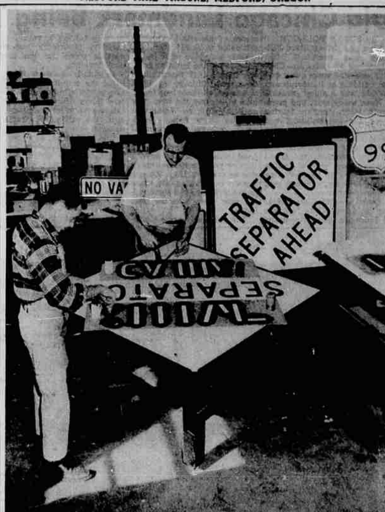
VARIETY OF WORK—The stenciling room in the Salem sign shop of the Oregon state highway department turns out a wide variety of work. Henry Hatfield, left, and John Helt work on a 48 inch by 48 inch traffic sign with black lettering on a light-colored reflectorized background. Signs are designed to give the greatest visibility, day or night.—(Oregon state highway department photo)
