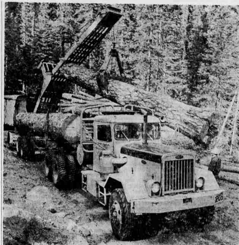
SELDOM SEEN —A logging truck the public sees, this specially built rig hauls up to 50 tons of logs, far in excess of public highway limits, over a private logging highway system operated by Brooks-Scanlon Lum-
