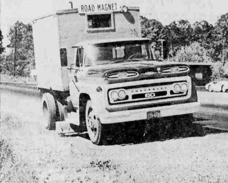
ROAD MAGNET —The Oregon state highway department's road magnet cleans Highway 99E, eight miles north of Salem. The magnet covered more than 6,000 miles of Oregon's highways last year, picking up three pounds of metal per mile.
