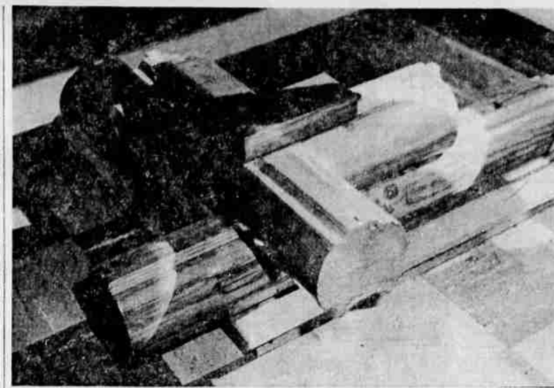
CORNER ASSEMBLY—A corner of an Alpine Log structure is assembled in the office to show customers how they fit together. All are interlocked so no air can get through. The logs are sealed with an asphaltic cement on all horizontal joints and at the joints at vertical corners. The company plans to change the log pattern so the logs are flat on the inside. This should eliminate dust-catching surfaces, Owner-Manager Norris Porter explained.
