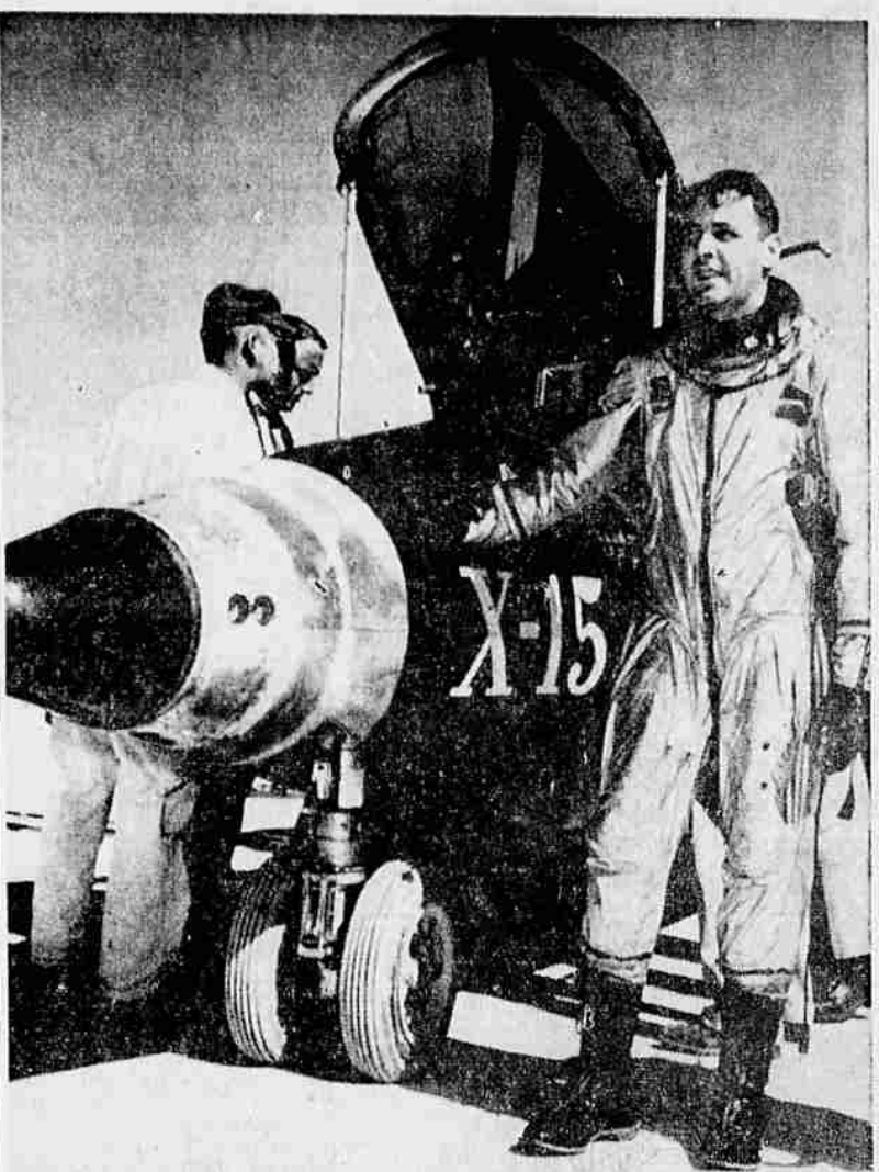
BREAKS SPEED RECORD — Maj. Robert White stands beside the experimental X-15 rocket plane at Edwards Air Force Base, Calif., after flying the craft at 2,905 miles an hour for a new speed record. The thermal paint on the nose of the plane is shown blistered by the heat. It at first was figured the plane reached a speed of 2,650 miles an hour but the faster speed was determined after further analysis of flight data. See story on page 2. (UPI Telephoto)
