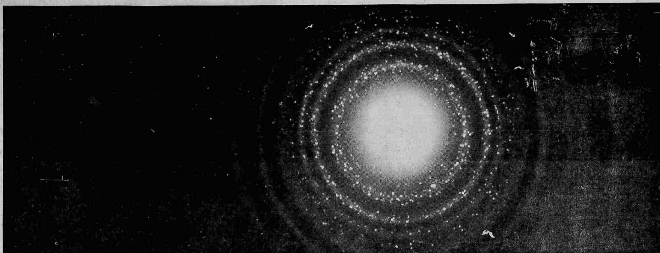
Circular pattern identifies deposits scraped from combustion chamber. It tells researchers many secrets. To get this pattern, deposits are ground up and placed above a film. Electrons are beamed directly at the deposits. The
