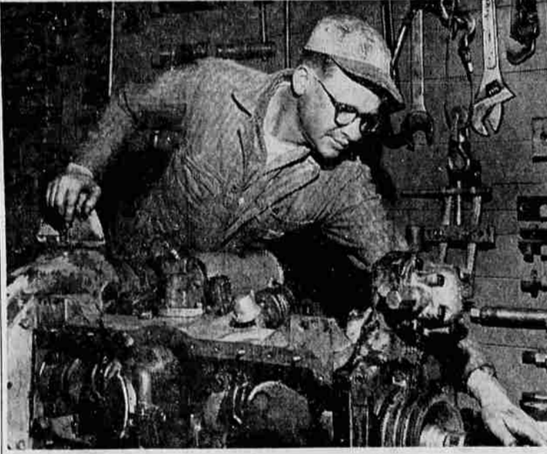
TURNS CRANK SHAFT — Derrald Sykes, new mechanic in the county shops, turns the crank shaft in a large engine so he can check the timing. Behind Sykes is a complete array of hand tools and small parts used in his work. Neatness and orderliness is emphasized in the shops for both safety and efficiency purposes. Equipment is carefully lined up outside the shops in the parking area when it is returned. Much of this winter's work is on routine overhauls to prepare it for intensive work next spring and summer.
