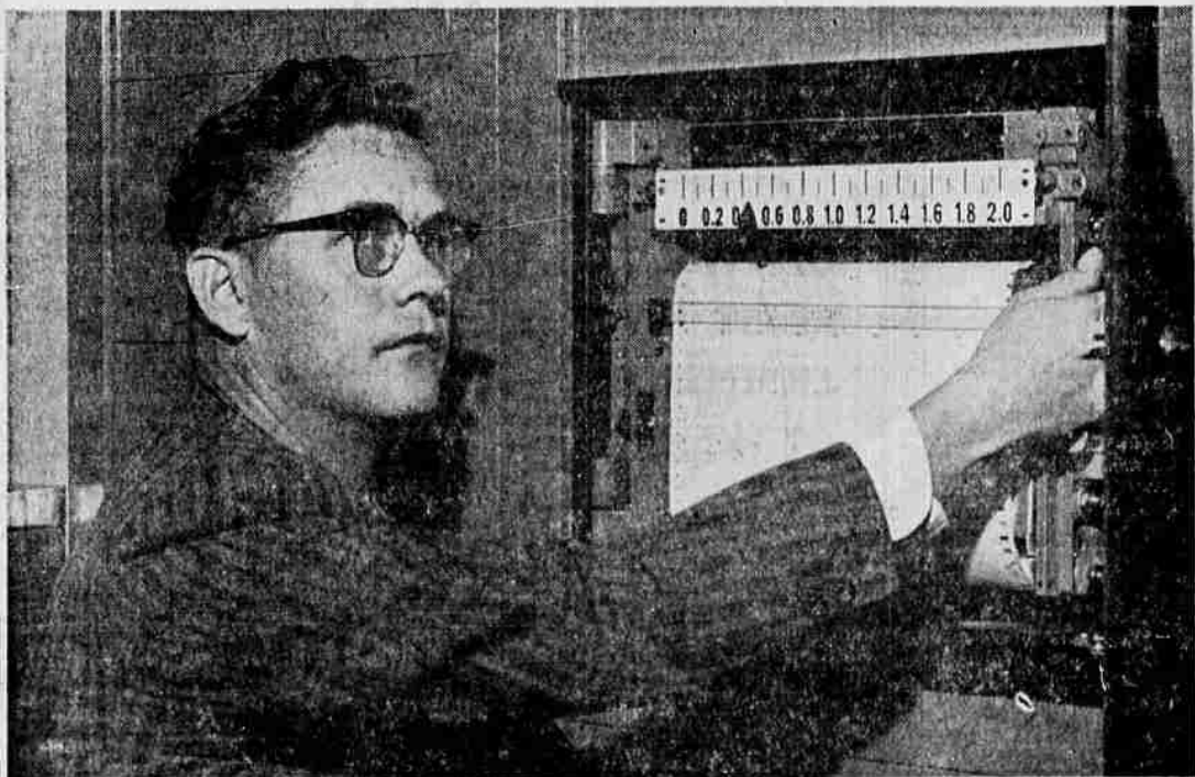
The device shown here is known as a solar radiation recorder. Pictured checking the machine is Herb Hove, a rawinsonde specialist. Twelve men are on the staff of the station, and they rotate shifts in order that each man takes his turn at night work. Eleven were at the station Tuesday and the twelfth, Robert Pentney, is on vacation. Ted Wiley, an electronic technician, is assigned to the station to keep the equipment in good order.
