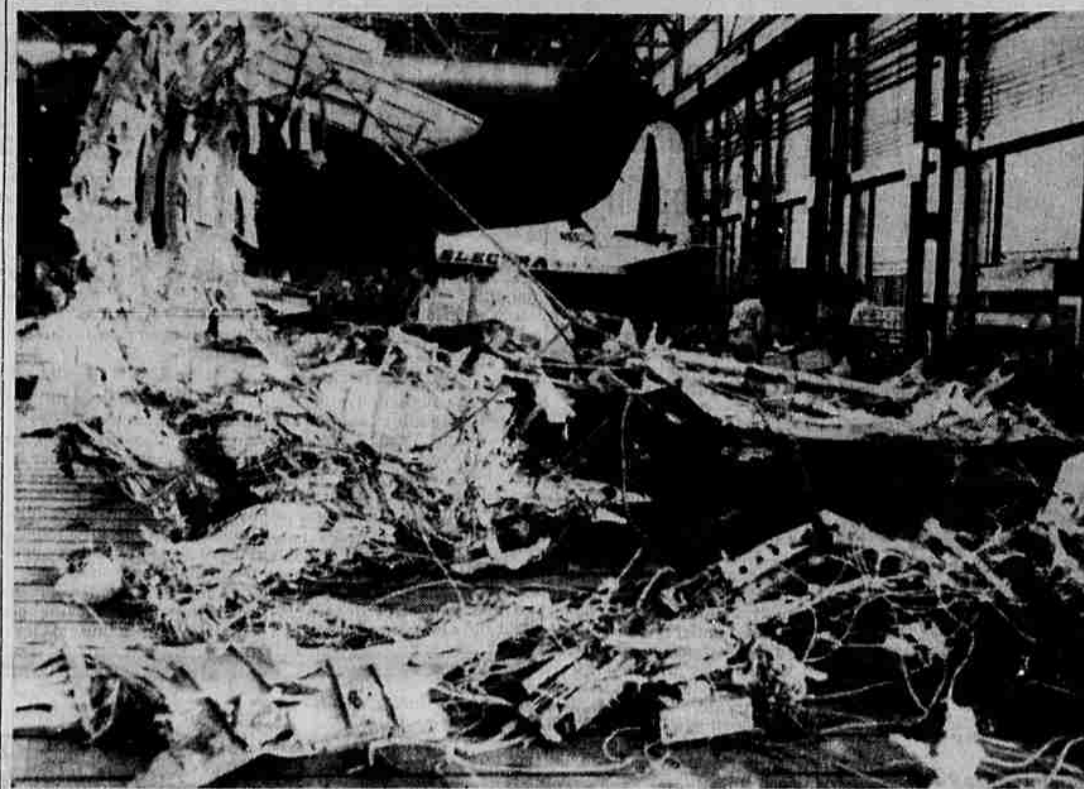
WRECKAGE REASSEMBLED - Parts of the Eastern Airlines Electra that crashed in Boston harbor Oct. 4 are being brought to a huge building at the Hingham Industrial Center at Hingham, Mass., and laid out in their original relationship to the plane. In this way investigators will seek answers to the crash which cost 62 lives. (UPI Telephoto)
