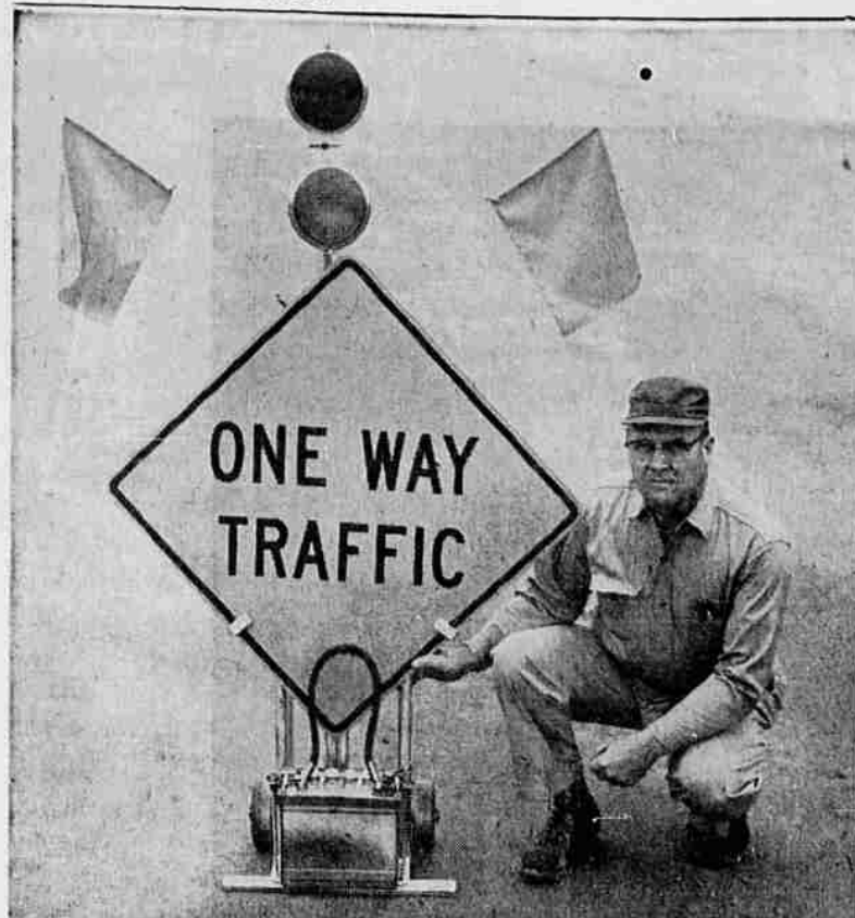
'FLASHING FLAGMAN' —A new portable light stand, known as the "flashing flagman" is now being used by the state highway department bridge and road crews to direct traffic while emergency repairs are being made. Shown with the development is Charles E. Flanagan, foreman in Portland for the highway department, who suggested the idea. The signs, under development for the past year, feature flashing red and
