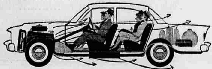
Front Engine... Passenger compartment exposed to engine noise and heat.
