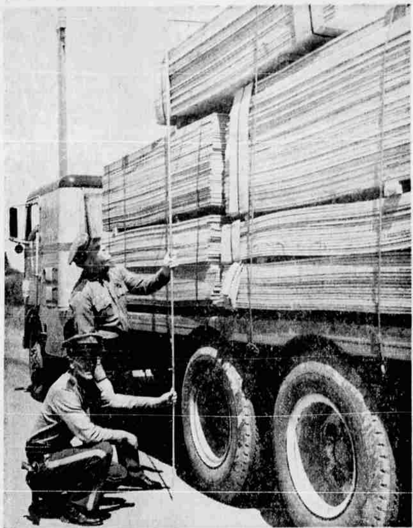
LOAD HEIGHT —Police recruits Dennis Daley (kneeling), Eagle Point, and Louis Brandt demonstrate how the height of a loaded truck is measured with an "L" shaped gauge. State police officers do not man the
