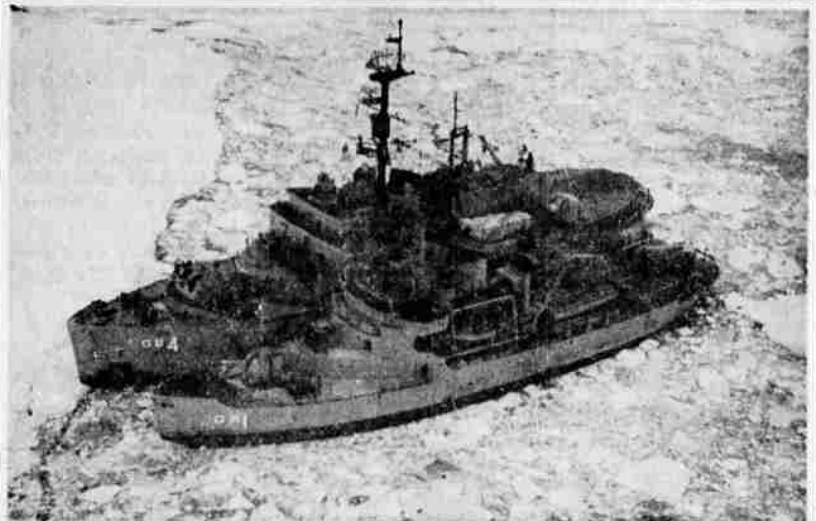
ON EXPEDITION —The two U. S. icebreakers which penetrated the heavy ice packs of the unknown Bellingshausen sea during Operation Deep Freeze 60. The larger ship, the USS Glacier, has 21,000 horsepower diesel-electric engines, the smaller USS Burton Island has 10,000 horsepower. Both ships carried scientists for oceanographic, geological, meteorological and topographic studies in the new area of Antarctica.
