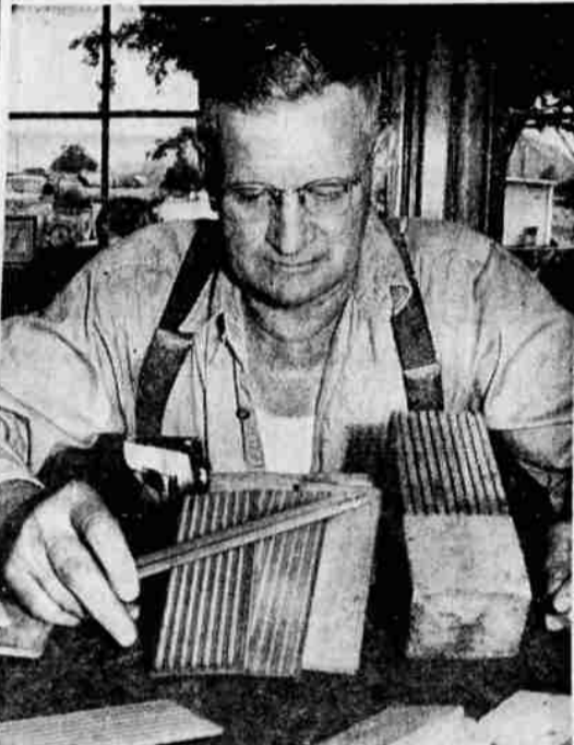
ILLUSTRATE STEPS—Illustrating steps in pencil making, Bernard Parent, manager of Gulf Red Cedar company, Central Point, shows section of incense cedar cant, at right, which has been sawed to make pencil "slats." At left are slats that have been grooved to make pencil halves. With lead in place, two slats will be glued together, then cut into eight pencils. —(AFPI Photo)
