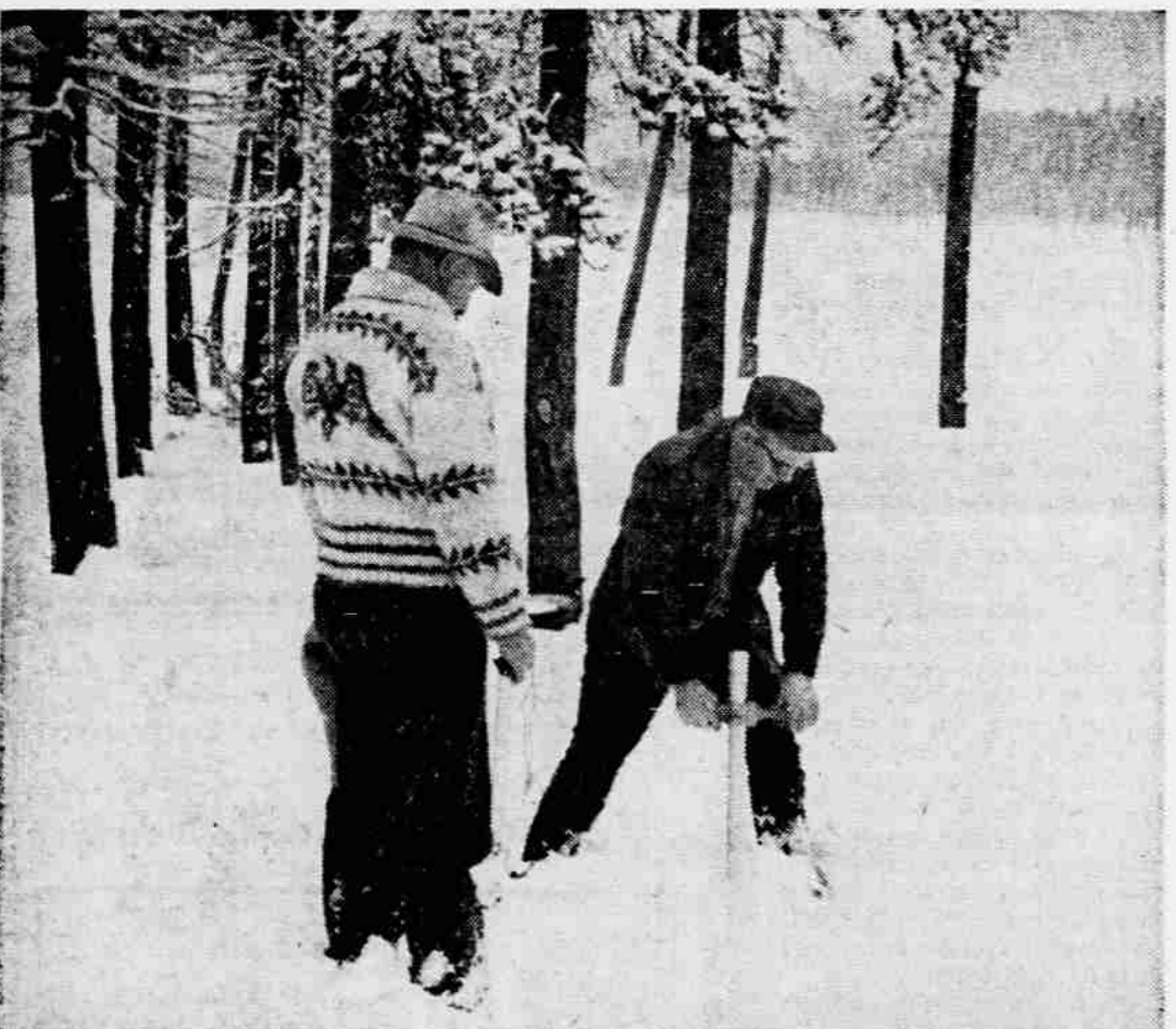
SINKS TUBE —Hoffbuhr, right, pushes tube into the snow to draw out a core at the Fourmile lake snow course. Some indication that the tube reached dirt must show after it is extracted. If there is more than a
