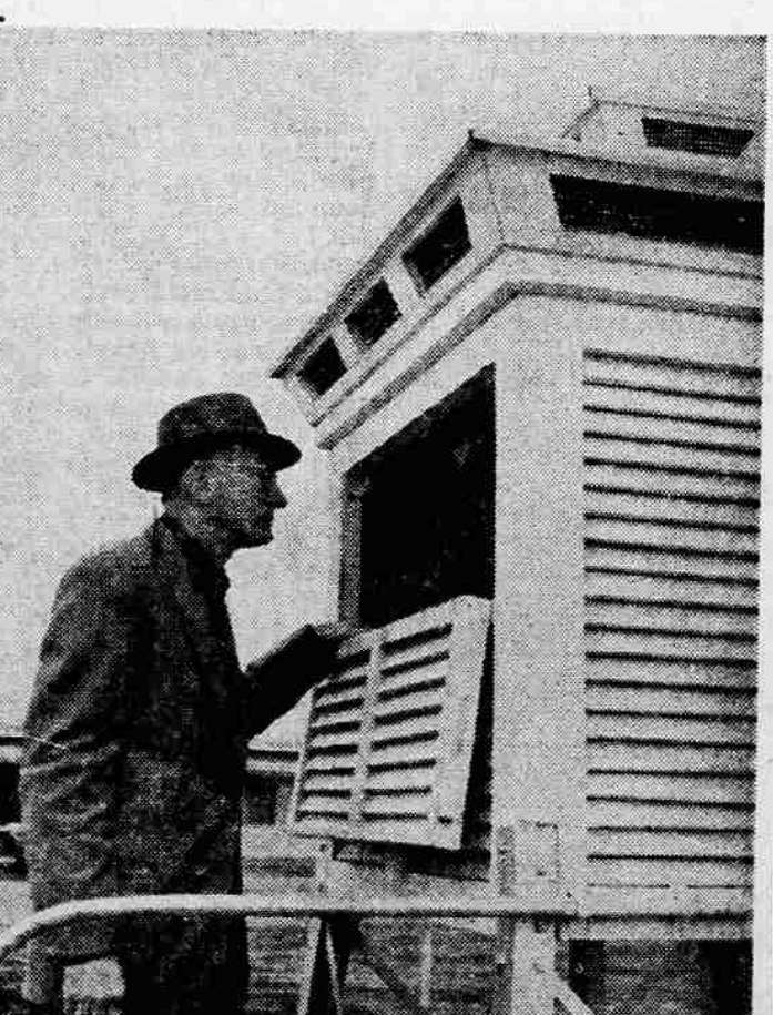
READS THERMOMETERS —Bob Church, above, head meteorologist at the Medford weather bureau station, takes the wet and dry bulb thermometer readings to determine dew point and humidity, part of the information needed in determining forthcoming weather conditions.
