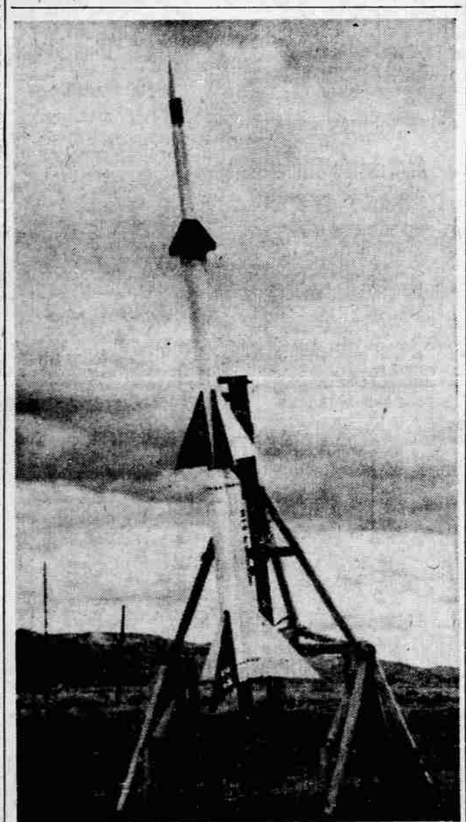
VELOCITY RECORDS BROKEN —Velocity records for a ground-launched missile, the HTV-2 shown on launching pad, have been broken by a mach 10 hypersonic rocket which reached a velocity of nearly 10 times the speed of sound within 10 seconds after launching. The three-stage missile was successfully test-fired last week and flew 6,000 miles an hour, according to Curtiss-Wright Corp., makers of the missile. —(UPI Telephoto)
