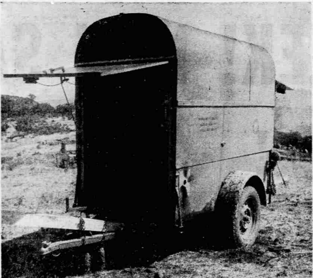
RADAR TRAILER —This OSC trailer is moved up to Roxy Ann butte or over to an Ashland location when hail researchers are notified of a thunder storm approaching the Rogue River valley. The trailer and equipment is manned by OSC students who use a movie camera attached to a radar scope to record radar's probe of the storm center. This and other data will help scientists determine what causes hail. The information will be used to alleviate or prevent hail damage to valley pears. This is sometimes the hail storm season for the area. Hail collectors and orchardists who wish to report storms are to call Jud Parsons, local head of the research program, at SPring 3-1060. This is a new number for Parsons' office.
