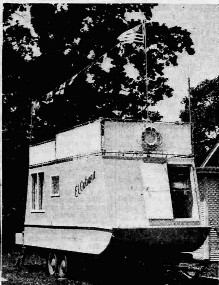
WATER HOME —This houseboat, designed and built by three valley men in their spare time, contains all the elements for luxury living, such as a modern kitchen, hot and cold running water, toilet, radio, refrigerator and sun deck. A 12-volt electrical system powers water pumps and appliances. The men, Don Paulsen and Don Kahl, Medford, and Larry Ruth, Ashland, will take turns using it with their families on week ends. The houseboat was launched this morning on Shasta lake, and will be taken on its initial cruise this week end. The hull is completely glassed, and, in spite of its seeming bulk, the boat draws only 4½ inches of water. It sleeps six.
