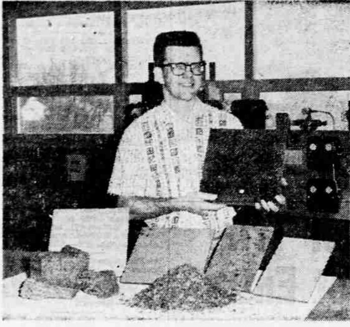
DISPLAYS BOARDS - Charles H. Burrows, wood technologist, displays experimental boards made from Douglas fir bark at Oregon's forest research center in Corvallis. Tree bark when ground into particles will form boards under heat and pressure without added binder. Burrows is holding one board made entirely of bark; other boards are overlaid with paper or veneer. Such boards may lead to a new industry based on the vast quantity of bark now burned at mills.
