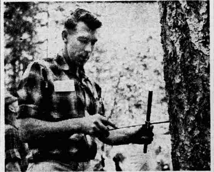
CORE SAMPLE —To determine the age of a tree and whether or not it shows prospects of becoming good saw timber within a reasonable length of time, core samples are taken with the device being demonstrated above by Calvin Smith of Industrial Forestry association, Medford. Width of the rings in recent years show if the tree is in a vigorous or slow stage of growth. If it has stopped growing the tree will be marked for removal when the area is logged.
