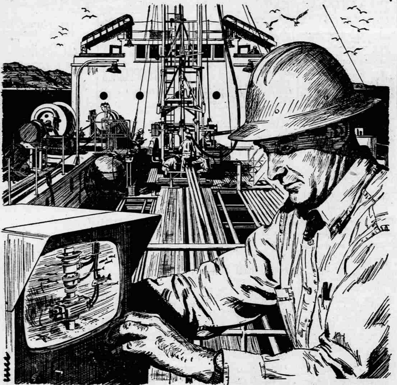
Navy landing ship converted by Standard for off-shore oil search. A 55-foot drilling mast is poised over circular 10-foot-wide opening from deck through bottom.
