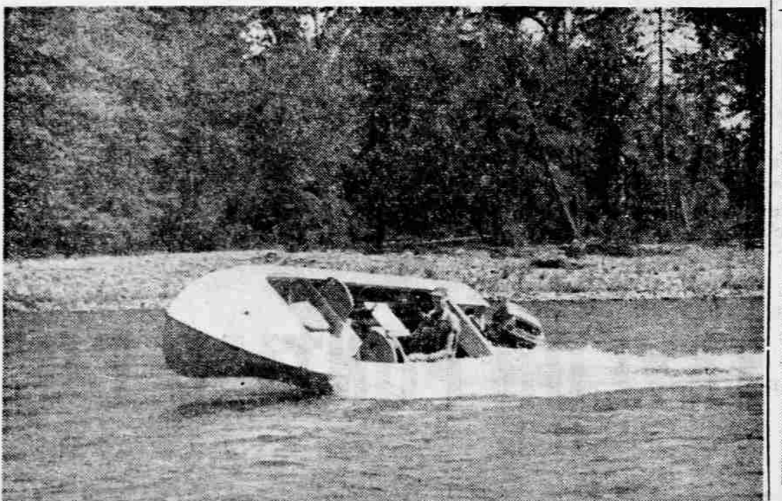
SHARP TURN —Going at a good clip into sharp turns above, boat builder Jim Allen lays a 15-foot Tru-V runabout over on its side until the gunwale touches the water. Powered by a 35 horsepower outboard, the boat literally jumps into planing position,
