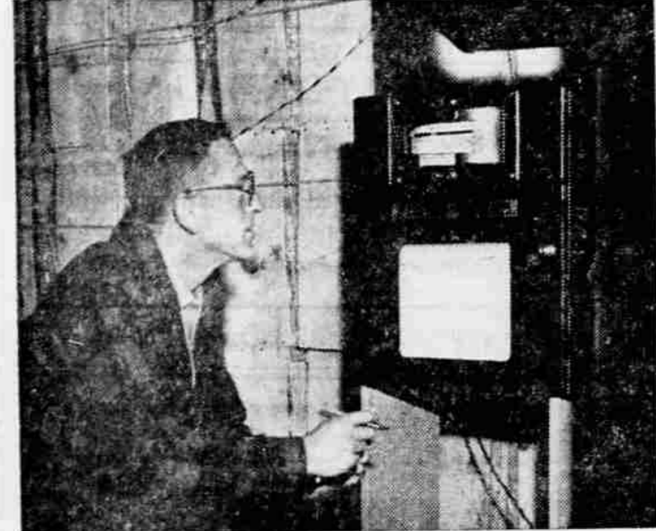
CHECKS TEMPERATURE —Don Root of Myron Root and company checks the temperature recording machine hooked up to the controlled atmosphere storage tent in the company's cold storage room. Thermo couples have been packed inside boxes of pears in five different locations inside the tent. The meter also measures the temperature in one location outside the tent. The purpose is to make sure the fruit is kept at nearly the same temperature. If there is a variety of temperatures the fruit at each of the five locations inside the tent will be checked for quality when they are unpacked.
