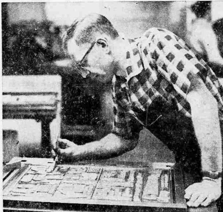
CHECKING TYPE —Lowell Sorenson, in the composing room at the Mail Tribune, checks a line of type in a full page ad that is being made up for an issue of the newspaper. The many pieces of metal that make up an ad are fitted into a steel frame, called a chase, which rests on a "turtle."
