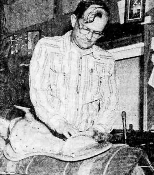
BIRTH OF A SADDLE—Proprietor Gibson scrapes the leather in the ground seat of a beginning saddle. The wooden form is a saddle tree, bought elsewhere. Leather parts are cut, soaked, and cased, then fitted and attached to the tree. About 15 to 18 pieces of leather make up essential parts.
