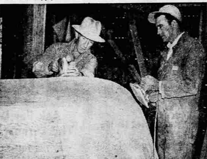
SANDING HULL —Above, co-owners Eldo Burgess and Leonard Wirz, are shown sanding the marine plywood hull of a 14-foot runabout being built in the Crater Craft boat factory in Ashland. The wood is finished to smoothness and all flaws are filled with a special hard bond wood filler before hulls are covered with fiberglass.
