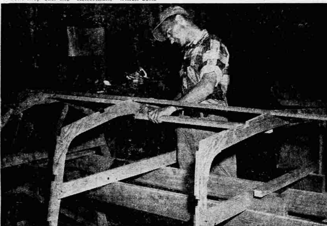
BOAT FRAMEWORK —Carl Surber, an employee of Crater Crafts, is shown above fitting a section of floor board filler in the framework of a 14-foot runabout under construction at the White Fir Lumber company, Ashland. The structural pieces are made of
