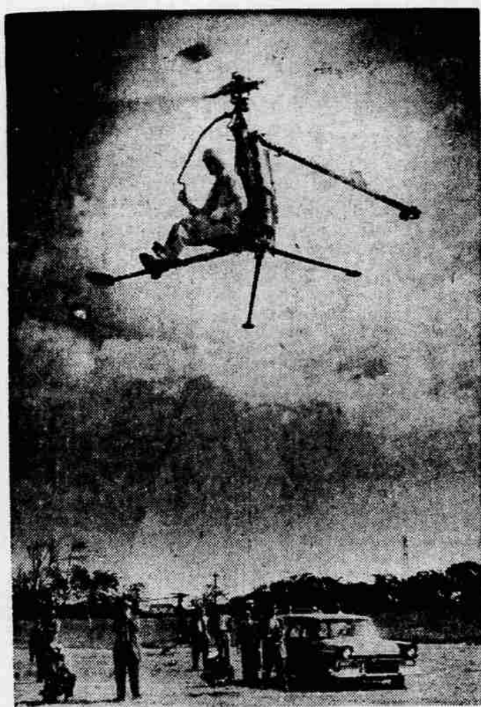
JEEP 'COPTER—Test pilot Richard L. Peck, 34, demonstrates the Marine Corps' new XROE-1 Rotocycle at Hiller Helicopters plant in Palo Alto, Calif. The 250-pound helicopter can be carried unassembled in the back of a station wagon or small truck. The Marines will use it for observation, liaison, rescue and unit tactical maneuvers.
