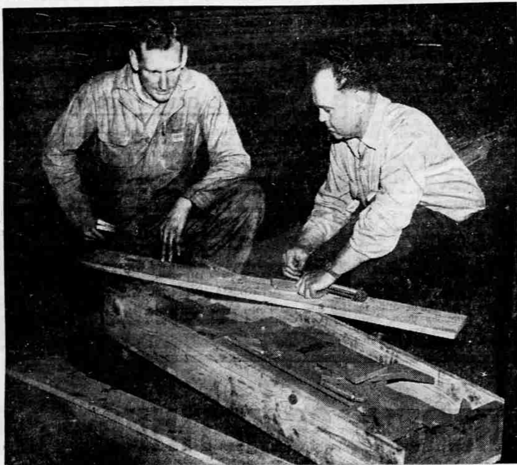
NEW TYPE "DOG" —Larry E. Juniper, right, owner of Pacific Machinery company, Medford, isn't complaining because his business has gone to the "dogs" lately. Juniper recently developed a new type sawmill carriage dog which is such an improvement over the old type that he is getting orders for them from sawmills along the Pacific coast. The air-operated units are manufactured by Pacific Machinery company, 1910 Table Rock rd. One of the advantages of the air tong dogs, as they are called, is that they grip the log better and minimize defacing of the wood, Juniper said. Juniper is shown above with machinist Roger Kornstad as they inspect one of the dogs that has been crated for shipment.
