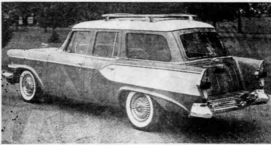
STUDEBAKER BROADMOOR — The 1957 Studebaker Broadmoor station wagon is a new body type for Studebaker as the company makes four-door models for the first time and expands its station wagon series to four models covering the low-price field. Engine choices range from 210 horsepower to 101 horsepower. The station wagons are almost six inches longer than last year. The four-door Broadmoor and four-door Provincial, along with companion two-door models will be shown Nov. 8 at DeLeigh Motors, 134 South Riverside ave., Medford.
