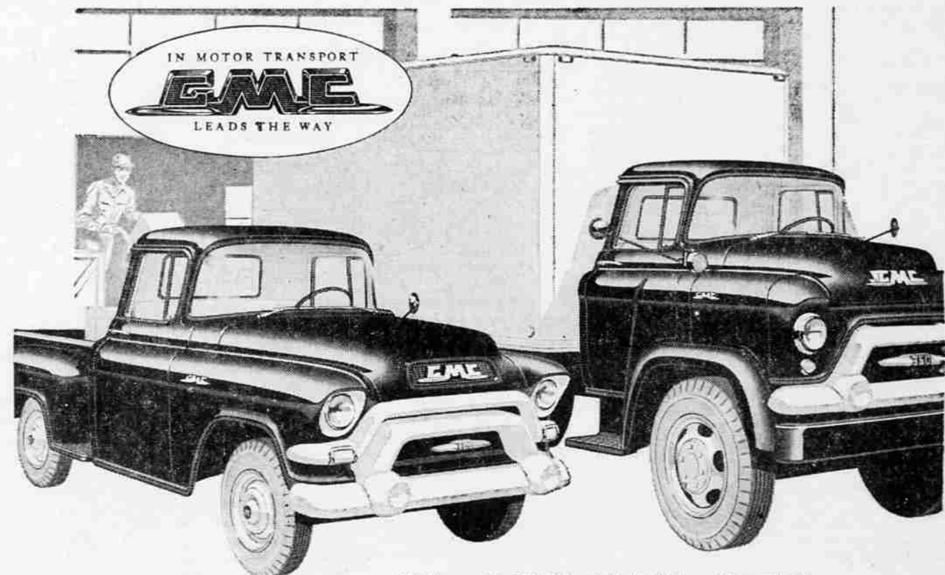
GMC shown at right is Model F550 fitted with 16-foot van. It's powered with a 140 h.p. six-cylinder engine—has over-size axles rated at 4,500 lbs. front 14,000 lbs. rear. It's designed for 18,000 GVW truck work. The smaller truck at left is GMC's popular 1/2-ton pickup with a 130 h.p. six-cylinder power plant.
