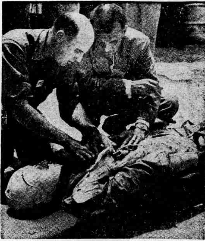
SAM WAS ALL BROKEN UP —Test pilots Bill Bridgeman (left), and George Smit view the battered "body" of Hurricane Sam after the dummy's parachute failed in a survival test at SMART rocket sled test site at Hurricane, Utah. Smith, only man to survive a supersonic bailout, said, "There, but for the grace of God, is me."
