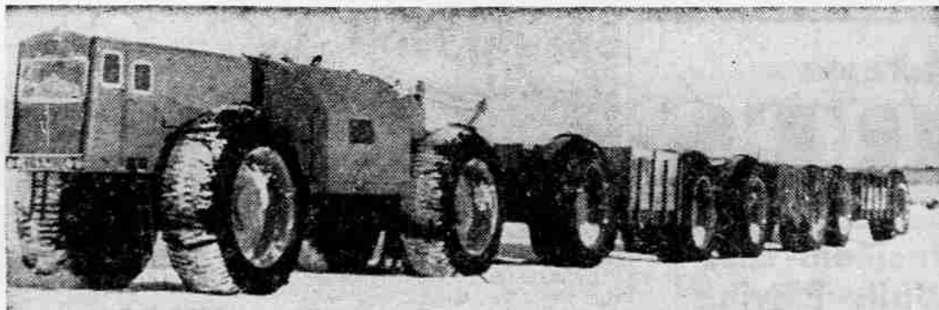
DESIGNED FOR ARCTIC, this is U. S. Army's new Sno Train now in service in far north areas. All wheels of cargo-hauling vehicle are driven by individual electric motors. Each unit shown carries approximately 12-ton load. (International Soundphoto)
