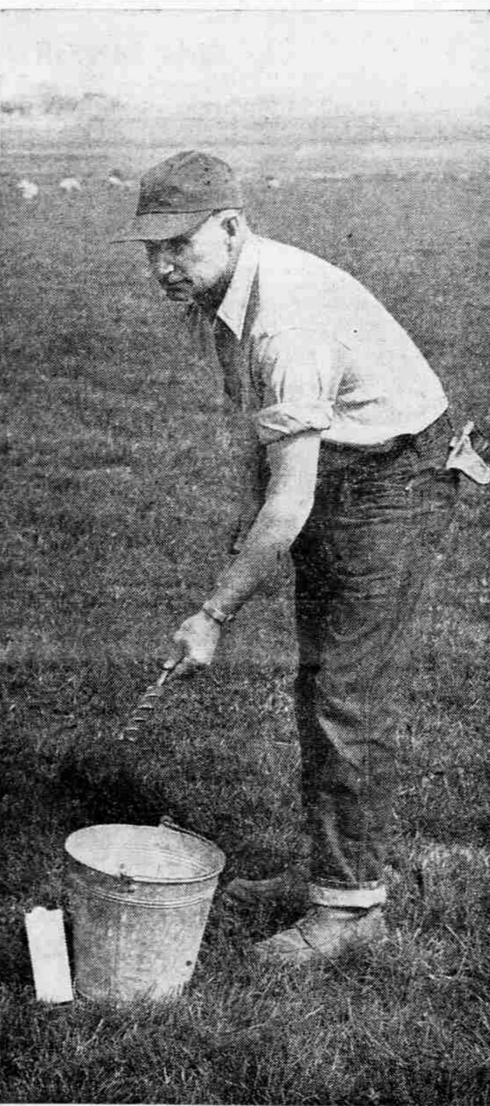
SAMPLING THE SOIL —John Niedermeyer, who farms about 200 acres between Medford and Jacksonville on Old Stage rd., uses the soil auger to extract a soil sample. Samples should be taken six or eight inches below the surface of the soil. The earth samples are then placed in a clean bucket, thoroughly mixed, dried and placed in the sample carton shown at left of bucket. The carton is then packed and sent to the soil testing laboratories at Oregon State college.
