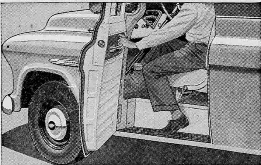
Watch your Step! Look for new CONCEALED SAFETY STEPS—an easy-to-see mark of a modern truck you'll find in new Chevrolet Task-Force trucks. They stay clear of snow, mud and ice to give you firmer, safer footing. You can see how different they are from the old-fashioned exposed running boards still used on some "new" trucks!
