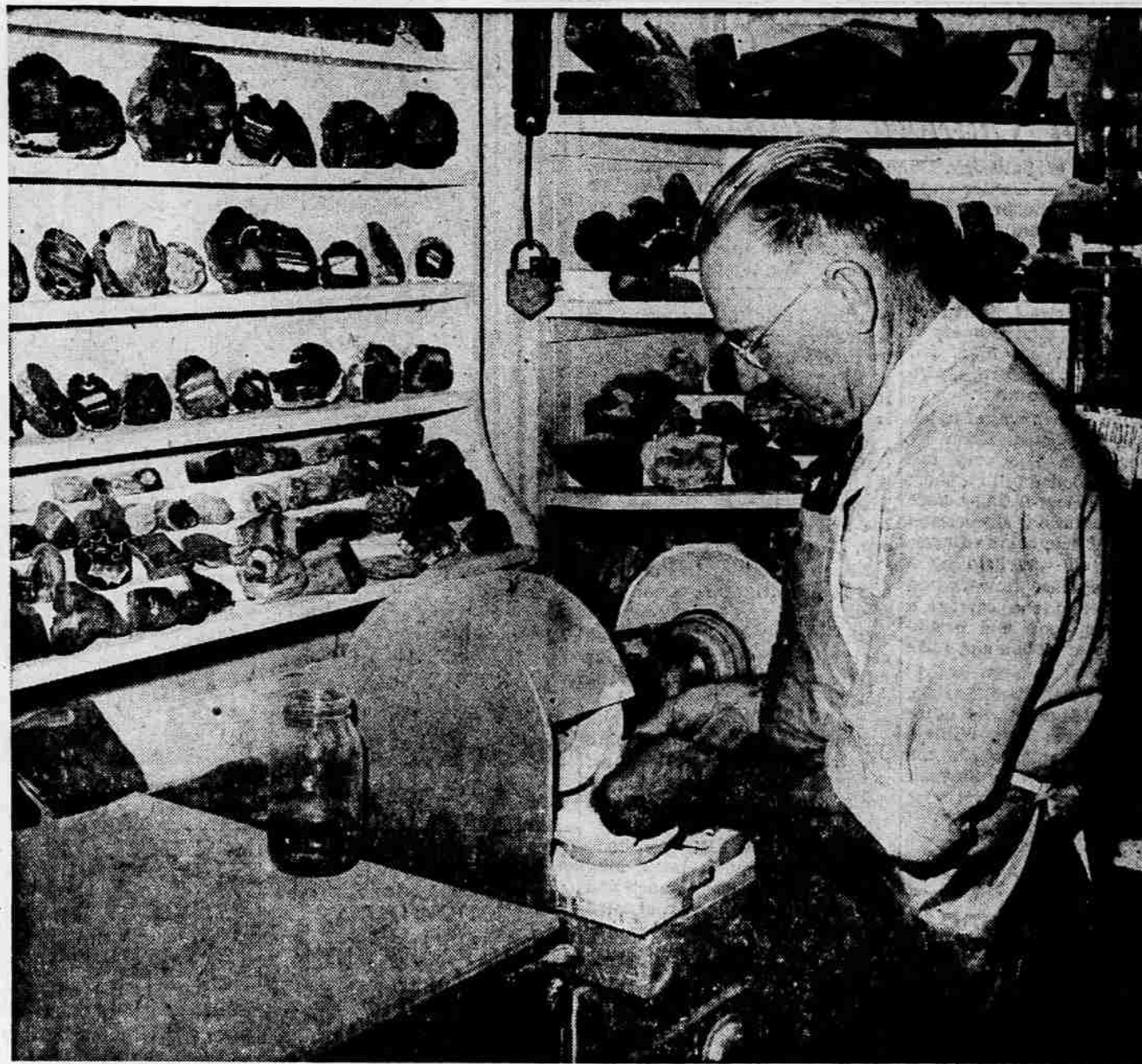
L. A. Mentzer is chairman of the coming show of Southern Oregon Gem and Mineral society. Mr. Mentzer, who has been collecting rocks and gems for 20 years, is shown here working at the polishing wheel made from layers of felt. Tin oxide is used as the polishing ingredient, and in the background can be seen some of the thunder eggs and pieces of petrified wood which Mr. Mentzer has cut and polished. The society's show is to be open from 10 a.m. to 10 p.m., June 18, and from 10 a.m. to 5 p.m., Sunday, June 19.
