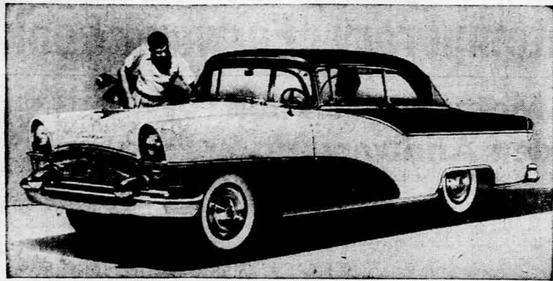
THE 1955 Clipper Constellation hardtop in Packard's medium priced line has a new 245-horsepower V-8 engine and revolutionary torsion bar suspension. The new type of suspension which eliminates conventional coil and leaf springs to provide a smooth, level, bump-free ride is introduced for the first time in a production car.
