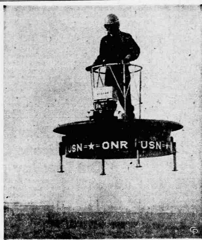
UNUSUAL AIRCRAFT, Navy's experimental "Flying Platform," achieves free flight with pilot Phil Johnston, Hiller Helicopter test pilot, aboard at Palo Alto, Cal. It is first aircraft using ducted fan for lift and propulsion to attain free flight. Pilot shifts weight to control horizontal flight. (International)
