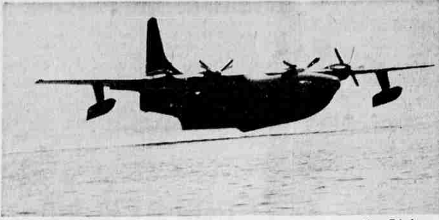
TEST FLIGHT —The Navy's new 60-ton patrol bomber, the XP5Y-1, takes off from San Diego Bay on its first test flight. The flying boat, which is hoped will be one of the answers to the submarine in event of war, has four turbo prop engines developing a total of 22,000 horsepower. The XP5Y-1 is expected to have a top speed of "more than 350 miles per hour," considered extremely fast for flying boats.
