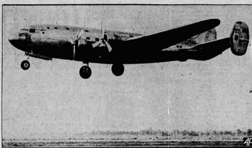
The new Douglas DC-4, world's largest commercial land plane is shown as it took to the air at Santa Monica, Calif., for its first test flight. Some 20,000 persons witnessed the flight of the 42-passenger plane, first of its type to be built for the nation's major air lines. The airliner cruises at 150 miles per hour.
