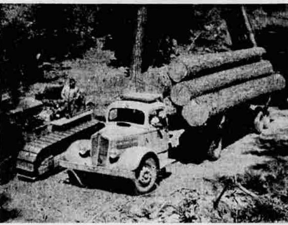
One of a fleet of White trucks and Isaacson Karry-Quad trailers taking out 7800 feet of logs on a private road operation.
