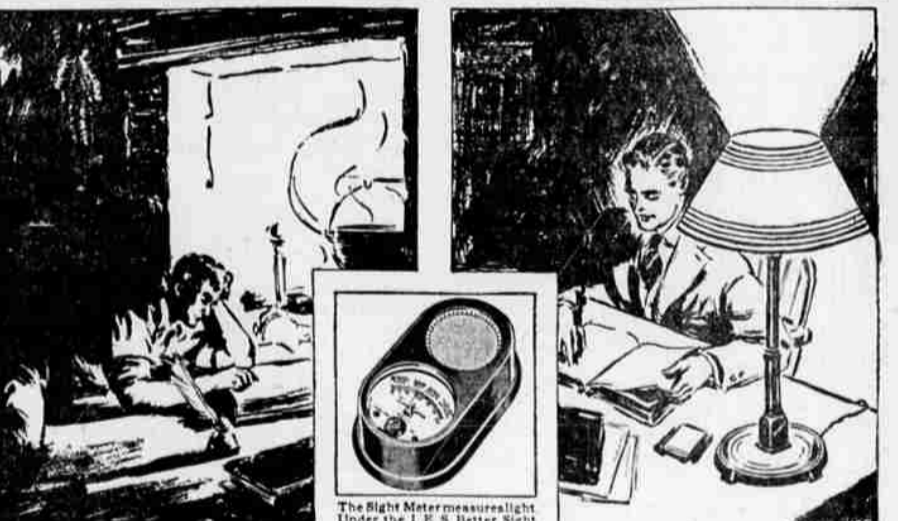
The Sight Meter measures light under the I. E. S. Better Sight lamp registers 20 to 30 foot-candles, the right light for studying
